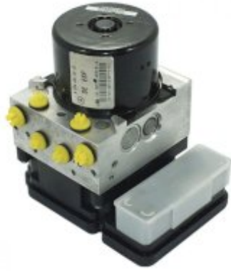
ESP KOMPLETE BOARD:25390 11600 PUMP:253431 0812
